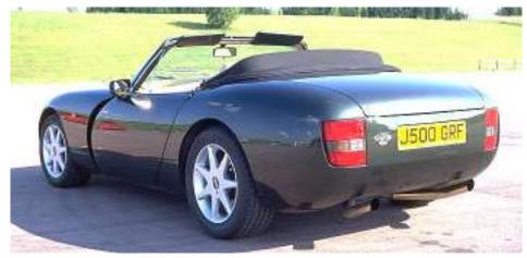
The Griffith 500 used the same body style but, with a 340 BHP 5 litre V8 engine under the bonnet, it was the answer to demands for the return of the Griffith and for even more power. The only external sign of the bigger engine is the 500 under the Griffith badge at the back and on the steering wheel.
